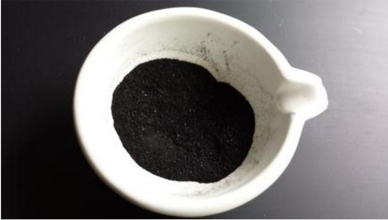
**Fig. A5.** Fine biochar power, final product after being pulverized.
